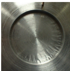
Figura 7.19. Aspect film PVAc (20, 25°C, 0.4, 0.8 m/s)
