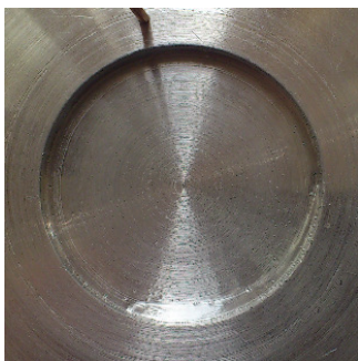
Figura 7.9. Aspect film PVA (40°C, 45°C, 50°C - 0.2, 0.4, 0.8 m/s)
