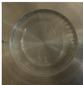
Figura 7.34. Aspect film CA (40°C, 0.5 m/s)
