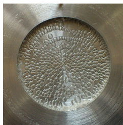
Figura 7.22. Aspect film PVAc (40°C, 0.4 m/s)
