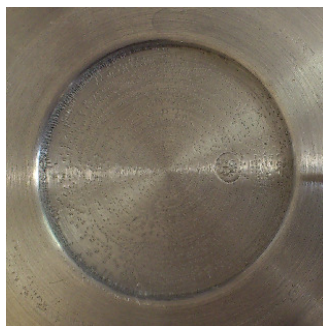
Figura 7.10. Aspect film PVA (60°C, 0.2, 0.4, 0.8 m/s)
